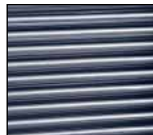
Closeup of bare tube condenser.
